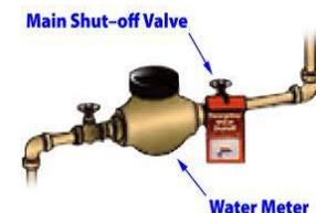
Example: Typical Water Meter, Shut-off, Valves, and Interior Plumbing
